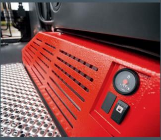
The main chassis structure has been coupled directly the counterweight structure, which is designed to absorb vibration; the steering axle is directly mounted into the counterweight by resilient cushioning, thereby absorbing travel shock and vibration.
