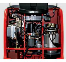
Moisture- and dust-proof motor AC drive technology incorporated in the new N 20/24 does not require any maintenance. Rapid and convenient access to all internal components is provided by simply removing the front service panel.
