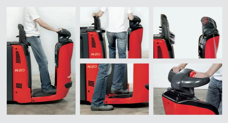
Access and platform Wide 390 mm entry on both sides and low 120 mm step-in height allow easy access to the truck. Absence of sharp corners and edges adds to operator safety and comfort. The full-suspension platform eliminates vibration. Its total area of 400 x 600 mm serves as a deadman zone and is covered with a soft, non-skid rubber mat providing highest standing comfort.
