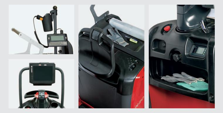
Working station Options include: Alternative load backrest height Rotating clipboard On-board terminal mounts on: Pole Load backrest Front bow Inching buttons are located on both sides of the truck for forward and reverse travel at 4 km/h.
