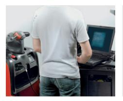
**Can bus connectivity** All truck data is immediately accessible for the service engineer by plugging into the on-board diagnostic port at the front of the truck. Setting parameters, troubleshooting and preventive maintenance are carried out quickly, easily and on time.
